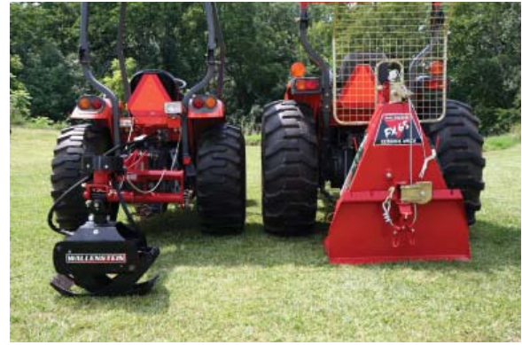
Figure 9. Examples of a 3-point mounted grapple and a 3-point mounted winch for safely moving logs. The tractor on the right is shown with a metal grill.
