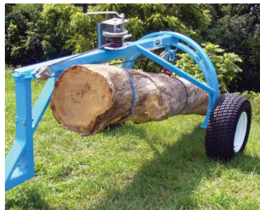
Figure 8. A log arch, fetching arch or sully lifts the end of the log being dragged to keep it from digging into the earth, rocks, roots, or stumps.
